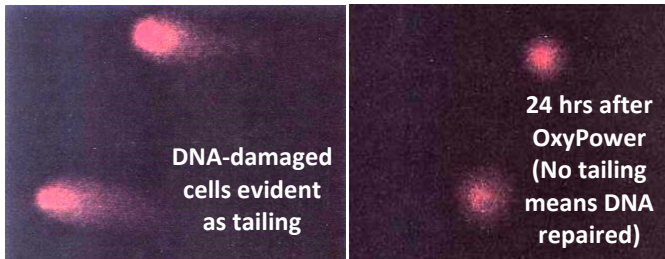
Comet Assay using electrophoresis under a microscope
